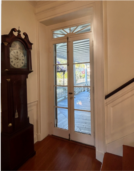
Heavy and tall objects near stairways and exit doors should be secured with straps attached to wall studs.
