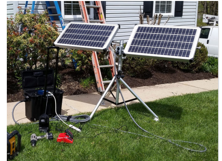
When charged, portable, solar powered backup batteries can be deployed in an emergency. (Example from Solar Stik)
