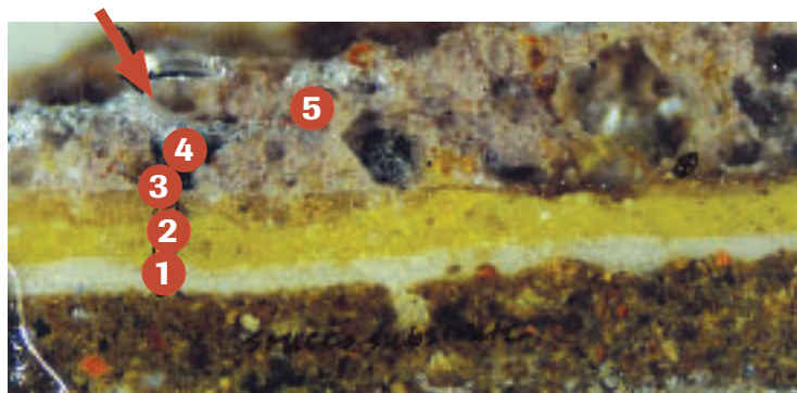
Figure 1 This cross-section image at 100X magnification of an area of painted stucco on the exterior of the Aiken-Rhett House shows that the first coating on top of the brown stucco was an unpigmented limewash, followed by the yellow limewash related to the art gallery period of expansion. Patches of the degraded remnants of the most recent pinkish sandy coating were discernible on the house before it was repainted. The notations identify the paint generations.
