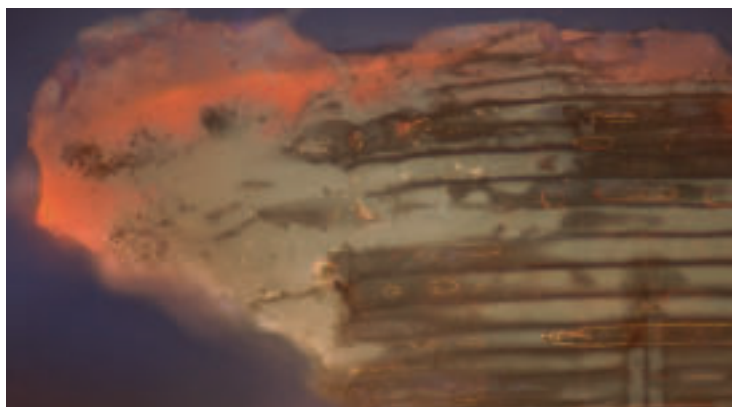
Figure 4 The cross-section sample from a protected area of carving on a Corinthian capital shows there is a degraded plant resin varnish trapped in the wood fibers (distinguished by a whitish autofluorescence color) with two more recent shellac layers on top of it (orange autofluorescent layers). The sample was photographed in reflected ultraviolet light at 200X.
