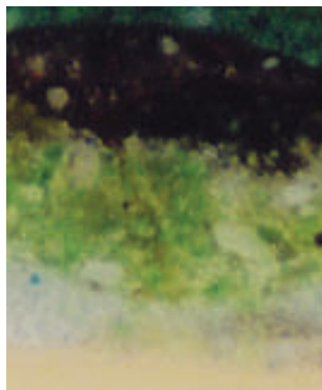
Figure 1 This cross-section image at 100X magnification of an area of painted stucco on the exterior of the Aiken-Rhett House shows that the first coating on top of the brown stucco was an unpigmented limewash, followed by the yellow limewash related to the art gallery period of expansion. Patches of the degraded remnants of the most recent pinkish sandy coating were discernible on the house before it was repainted. The notations identify the paint generations.
