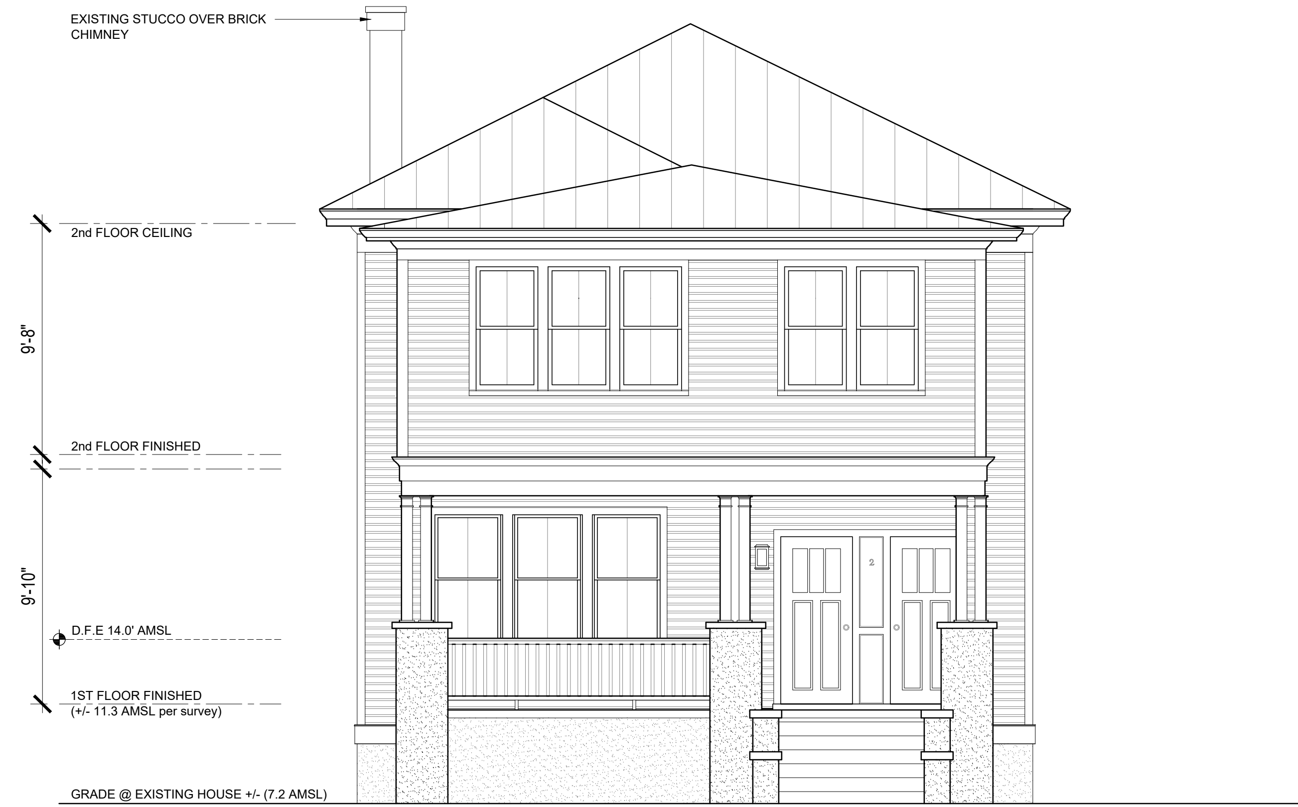
EXISTING SOUTH ELEVATION NO ADDITIONAL CHANGES REQUIRED
