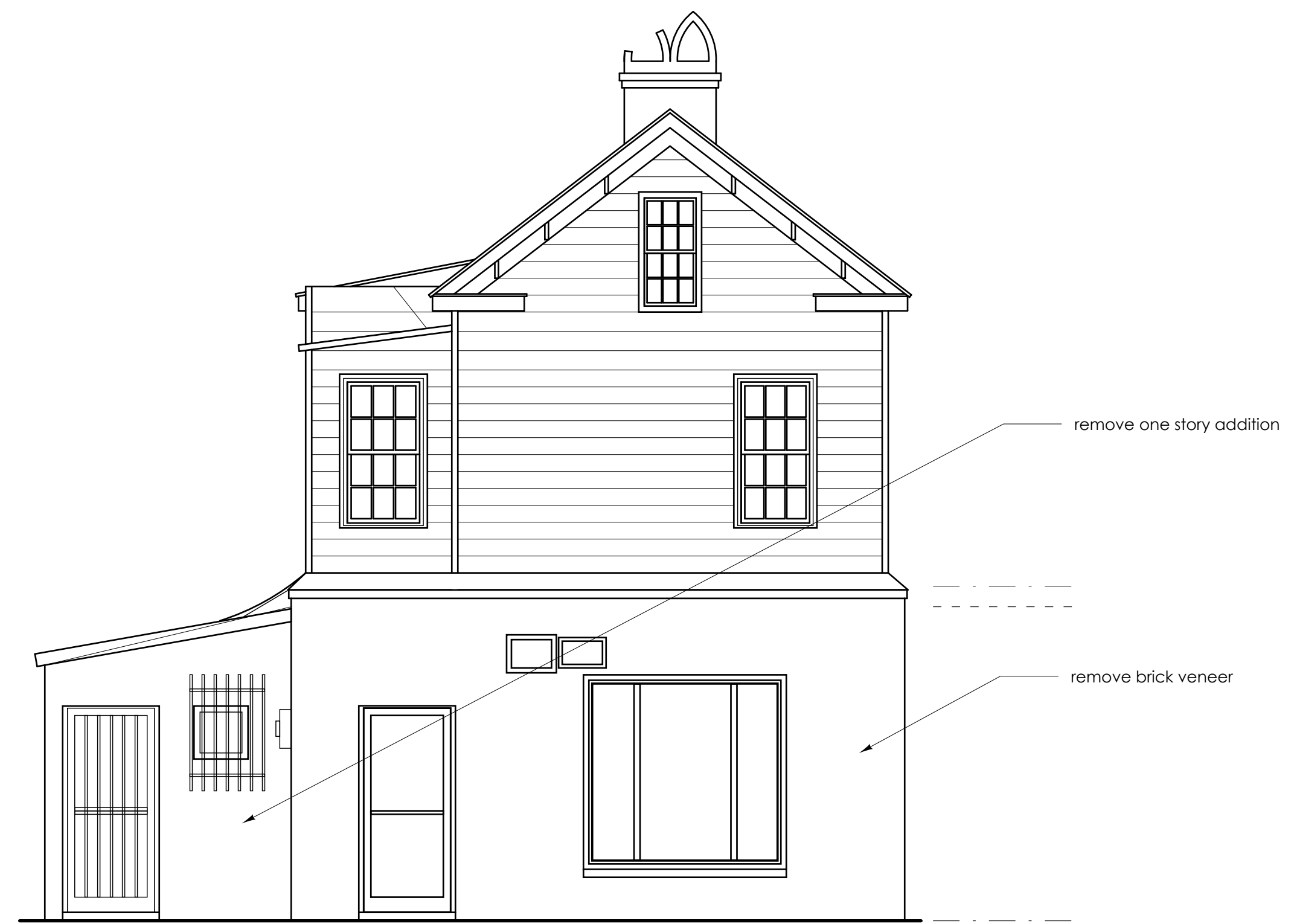
existing south (spring street) elevation: 1/4" = 1'-0"
