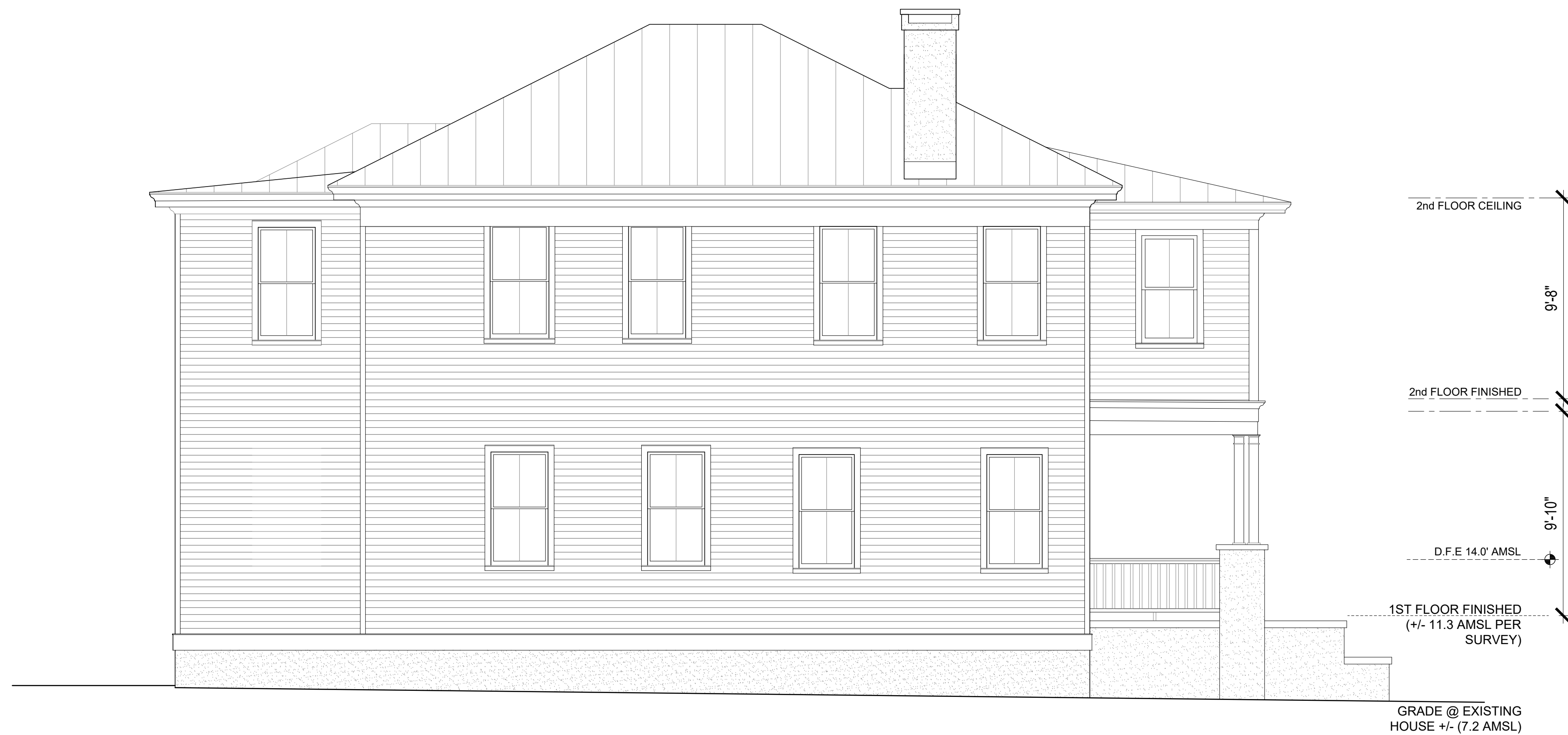
EXISTING WEST SIDE ELEVATION 1/4" = 1'-0" (1/8" IF HALF-SIZED)
