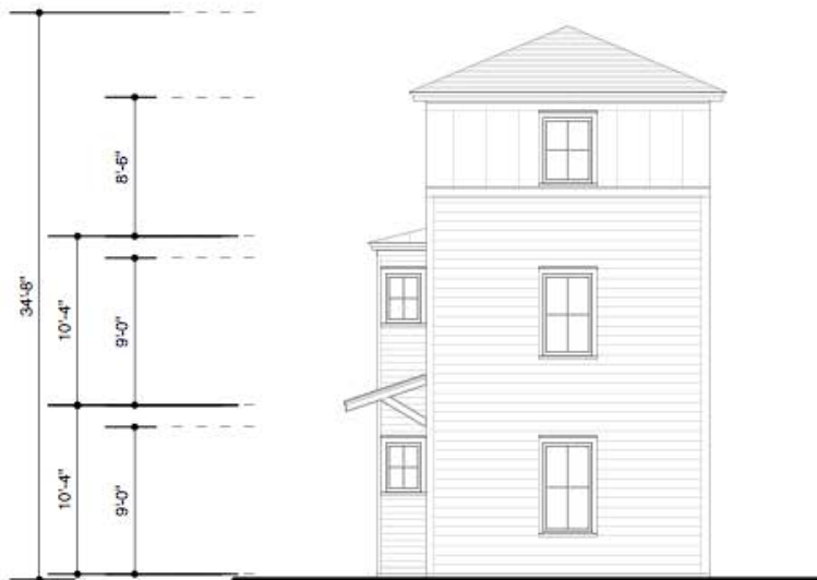
3 SMALLS ALLEY: SOUTH ELEVATION
