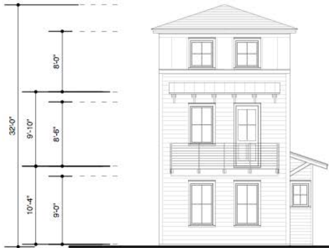
2 SMALLS ALLEY: NORTH ELEVATION 1/8"=1'-0"
