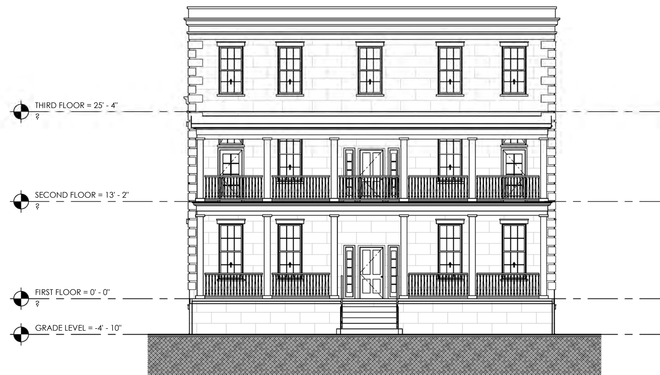
1 SOUTH ELEVATION EXISTING SCALE: 1/8" = 1'-0"
