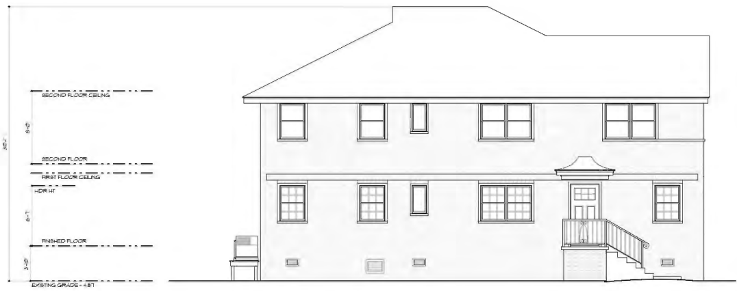
1 SOUTH ELEVATION - AS-BUILT A202 SCALE: 1/4" = 1'-0"
