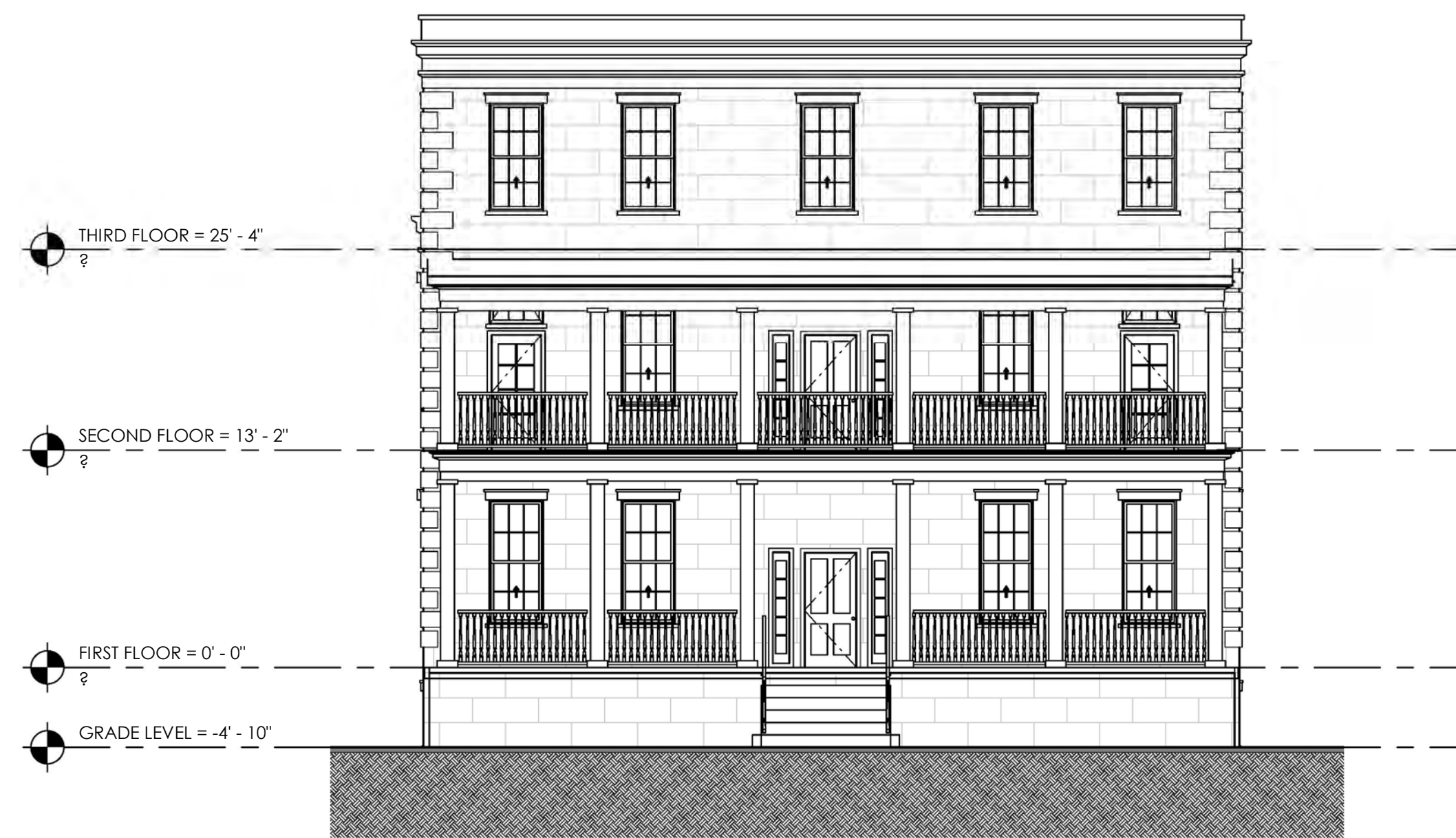
2 SOUTH ELEVATION EXISTING SCALE: 1/8" = 1'-0"
