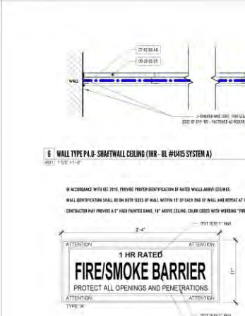
5 TYP. FIRE WALL/BARRIER SIGNAGE SIZE: 1 1/2"
