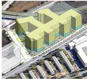
Residential uses are built over the parking and commercial spaces. Higher ceilings on the ground floor allow for varied pedestrian friendly uses.
