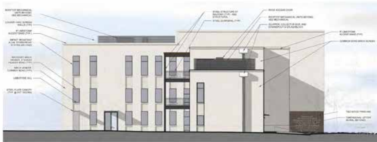
1 NORTH BUILDING ELEVATION: FINAL APPLICATION
