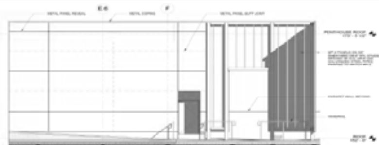
1 PENTHOUSE - ELEVATION @ MECH SCREEN
