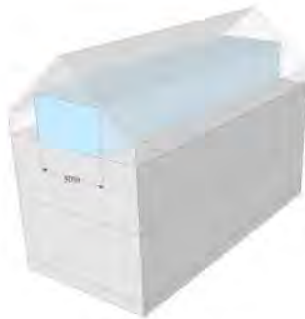
Gable Roof, no dormer Total footprint: 1,200 sq.ft Habitable space: 600 sq.ft (shown in blue) = 50%
