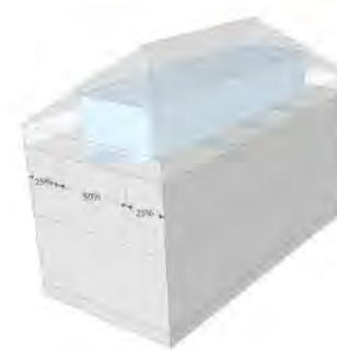
Hip Roof, with dormer (7) Total footprint: 1,200 sq.ft Habitable space: 594 sq.ft (shown in blue) = 49.5%
