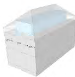
Hip Roof, no dormer Total footprint: 1,200 sq.ft Habitable space: 484 sq.ft (shown in blue) = 40.3%
