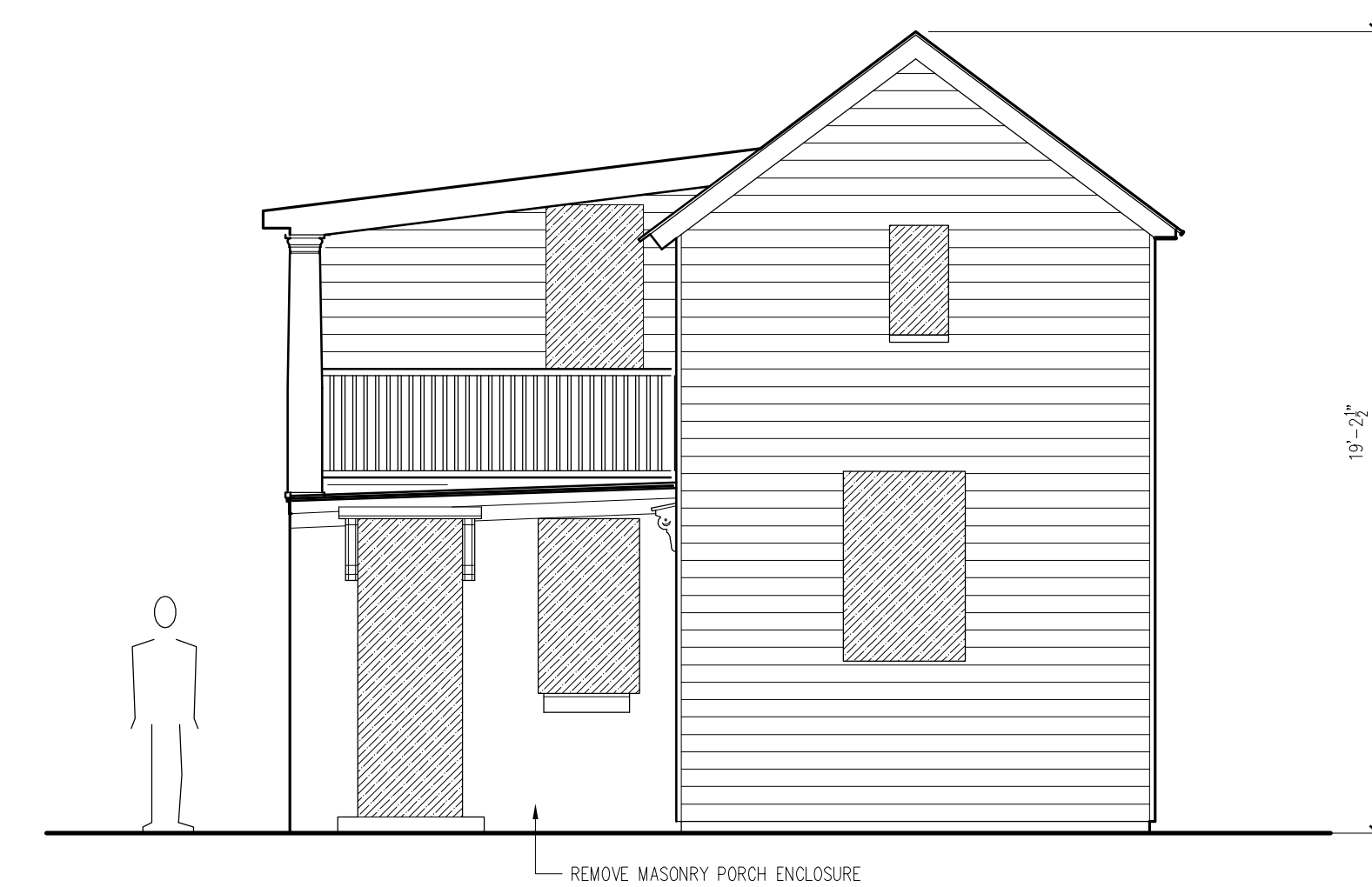
EXISTING EAST ELEVATION
