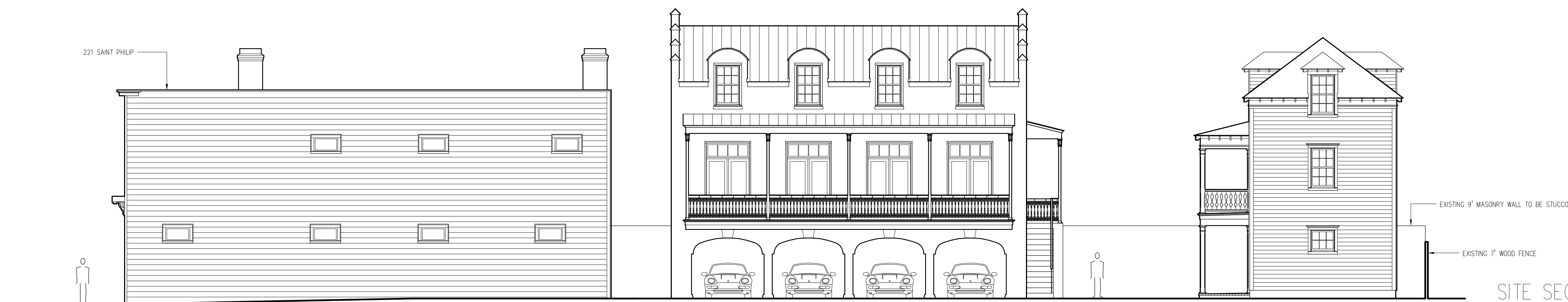
SITE SECTION LOOKING NORTH SCALE: 1/8"=1'
